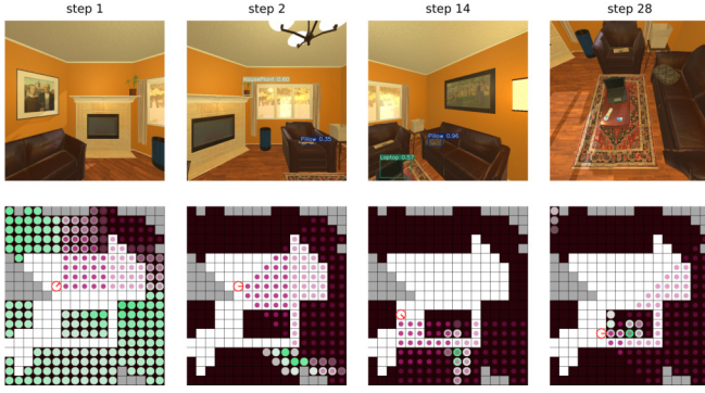
Fig. 3: Example Sequence. Top: first-person view with object detection bounding boxes. Bottom: Visualization of belief state corresponding to each view. See Fig. 2 for the legend of the belief state visualization. Our method (COS-POMDP) successfully finds a CreditCard in a living room scene, leveraging the detection of other objects such as FloorLamp and Laptop. For more examples, please refer to the video at https://youtu.be/RneTq4o0a-A .
