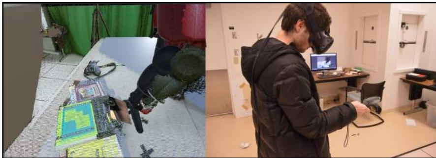
Fig. 1: Using ROS Reality, our virtual reality interface, to teleoperate a robot arm to perform a cup stacking task. The user is able to see a 3D model of the robot, an overlaid point cloud, and a camera feed from the wrist camera of the robot.
