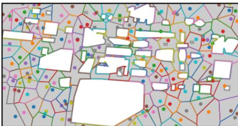
Fig. 3: **Map partitioned into Voronoi cells.** White holes represent regions containing landmarks.
